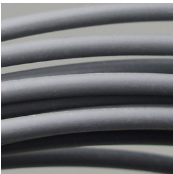
magnetic to magnets, filled with carbonyl-iron
