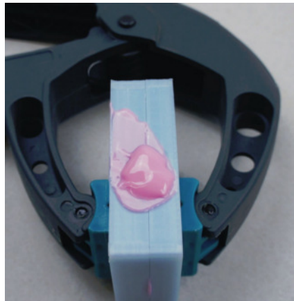
form printed from Moldlay (blue) filled with a 2K resin (pink)
