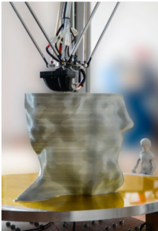
torso while being printed with a delta-printer
