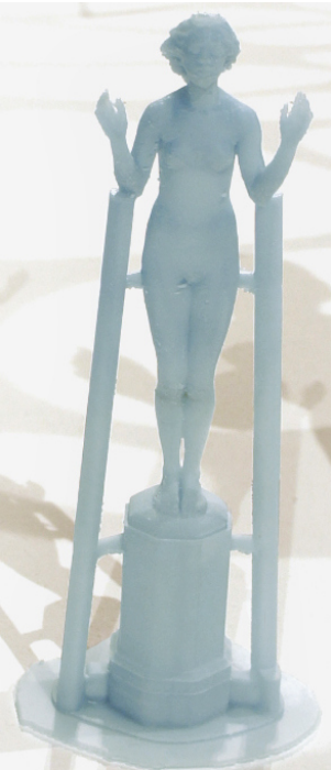
printed model with feeder and ventilation channels
